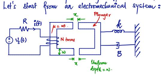
Consider the electromechanical system shown above. The plunger is attached to a spring (const. = k), and a dashpot (const. = B), where the spring is
